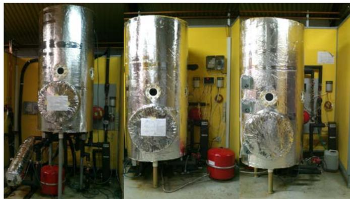
**Figure 2: Small smart solar thermal demonstration system Denmark (Source: DTU).** Three smart solar thermal combi systems have been tested and demonstrated at DTU. They use low cost electricity as backup energy. The upper picture shows the three collector arrays. The lower picture shows the three different variants of storage tanks tested in parallel.
